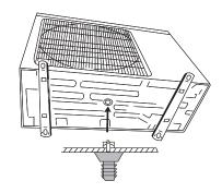
Drain Fitting Installation
