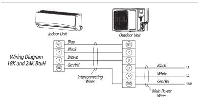
5. Following the same wire colors and terminal references from the indoor unit, tightly connect interconnecting wires to the outdoor unit terminal block per wiring diagram above.
